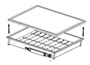
Remove 4 nos. screws from Diffuser Frame to open the Fitting for access.
